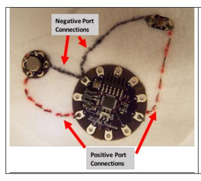
This circuit uses a button attached to pin 11 to control the buzzer attached to pin 5. The buzzer and button are grounded individually on the negative port.
