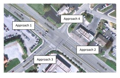
Traffic signals work by alternating the ability for vehicles to travel on each approach using different phases, which can have set or varying phase lengths. Phase lengths are the amount of time assigned to each green, yellow, or red phase.
