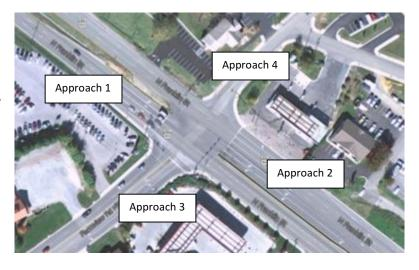
Traffic signals work by alternating the ability for vehicles to travel on each approach using different phases, which can have set or varying phase lengths. Phase lengths are the amount of time assigned to each green, yellow, or red phase.
